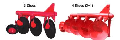
Used for deep ploughing in root-infested, sticky, stony, and hard soils. Mixes remains of crops and weeds throughout the depth of ploughing, hence ideal for rain-fed areas for checking soil erosion by water and wind.
