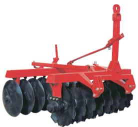
The Offset Disc Harrow has a heavier weight per Disc and thus has the penetration ability to break down large clods normally left after disc ploughing or Chisel Ploughing in hard grounds. It is of robust construction, used as mounted or trailed and ideal for chopping and mixing of stubbles and crop residues in the soils.
