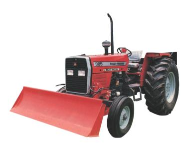
The Power Dozers are designed and built to match the performance of the Millat Tractors. They are operated hydraulically by single or twin double acting rams. The points of attachment of the dozer to the tractor are reduced to an absolute minimum and the mounting brackets, once fitted, can be left in position enabling the sub-frame and blade to be quickly removed and attached. The blade is fitted with a reversible and replaceable cutting edge of high carbon steel.
